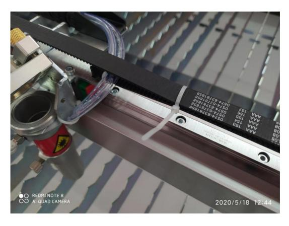
We level the machine. The level should be at least 400mm long. Make sure the tool you are using is in good working order! Place a level on the aluminum surface of the left side guide, then the right side, and make adjustments using the machine's leveling feet. After moving the machine to a new location, leveling must be repeated.
