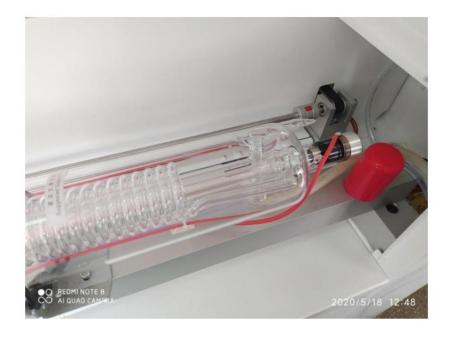
Turn the lamp so that the ebb for introducing water into the lamp, which is located near the red silicone insulator, is oriented down and the opposite one up. After this, remove the protective red insulator and connect the red cable, **put the insulator back on!!!** Connect the negative cable to the opposite edge of the lamp. We fix the lamp with clamping rubber bands, placing them on the hooks of the mounting prisms.
