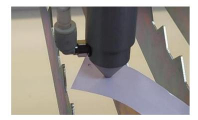
After gluing, press the "pulse" button. The removed tape should have a hole punched with a laser and an imprint of the spout outlet around it. The two circles should be one in the center of the other.
