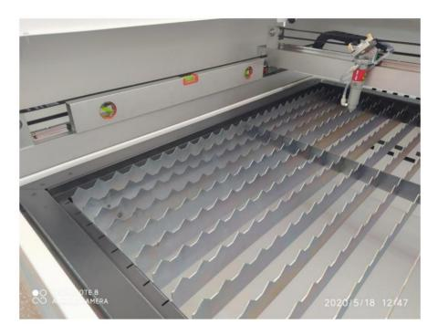
Installation of slats. We insert the lamellas into the machine table in accordance with the mark on the lamella (hole). All lamellas should be oriented with the mark in one direction.
