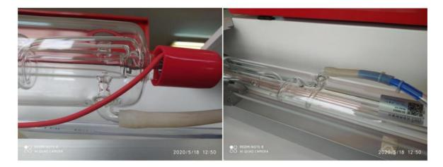
We connect the chiller. Fill the tank with enough water so that the coil is completely submerged. The cooling circulating water must be clean, free from dust and dirt. Next, connect the hose that goes from the pump to the water supply to the machine, and the free end of the hose to the discharge.
