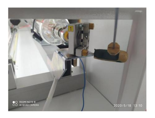
The upper screw reflects the beam up and down, the lower side one to the left and right. You should twist it carefully, little by little, so that the beam does not leave the target field. After adjustment, secure the result by tightening the brass nuts.
