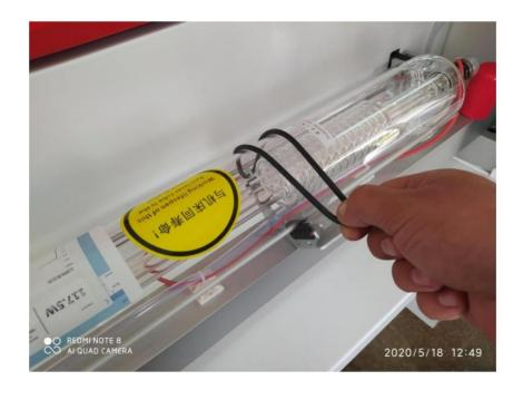
Place the water supply hose on the outlet that faces down, and the water discharge hose on the outlet that faces up.
