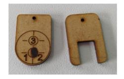
when hit by a laser beam it leaves a mark. When adjusting the laser beam, safety precautions must be observed. It must be remembered that the path of the laser beam must be inside the machine and not go beyond its boundaries.
